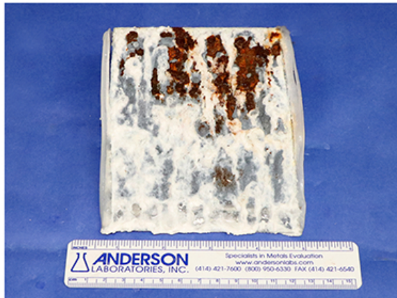
G235 Overbend (Tool Defects)
