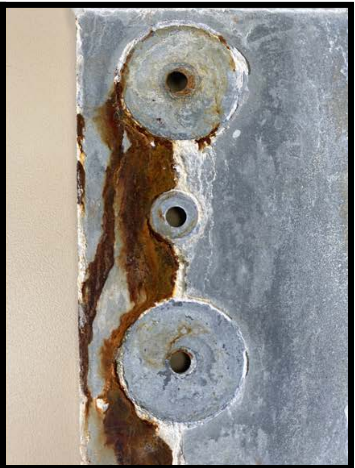
HDG VS. SS-CG315L-DFL, 960 Hours Exposure
