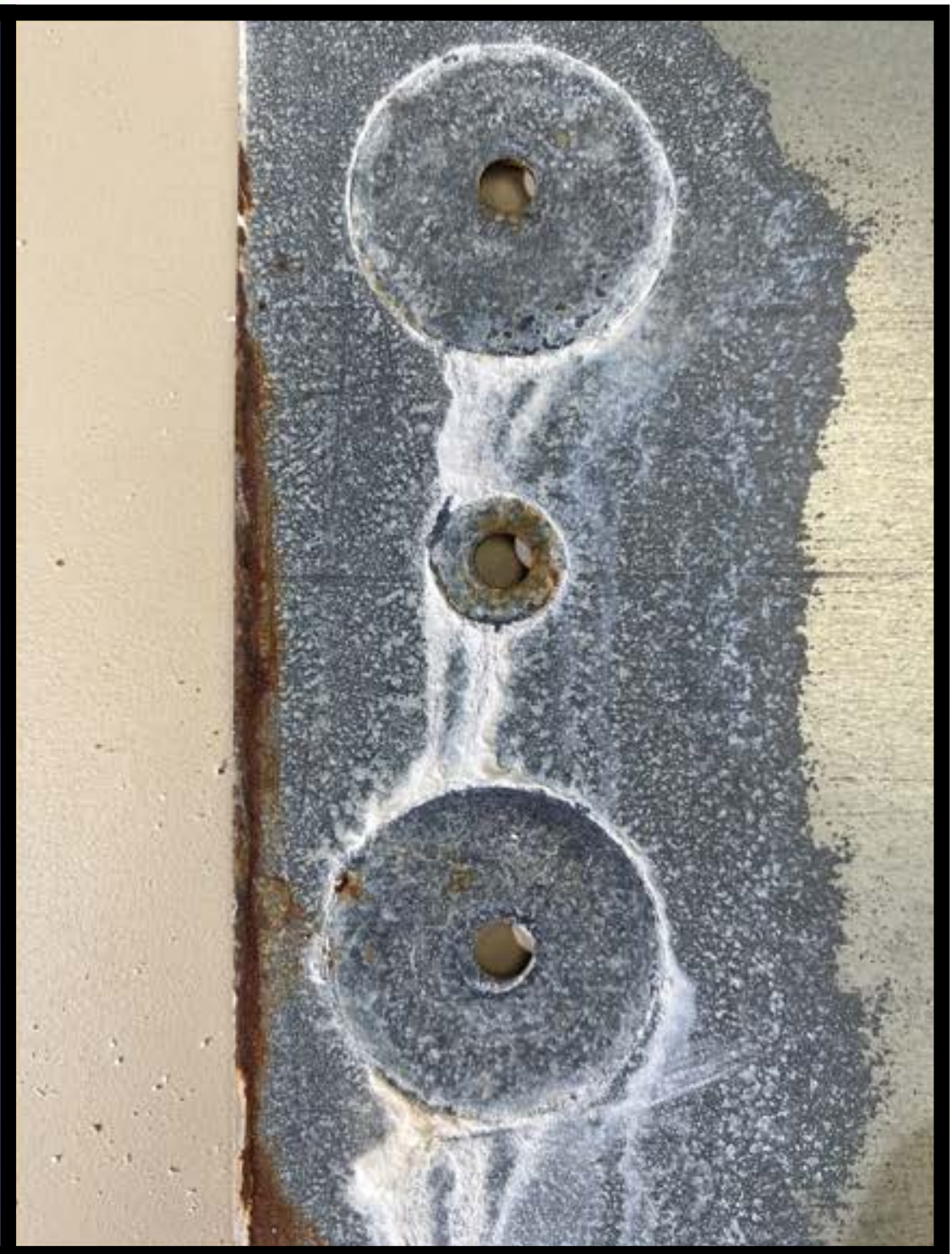
HDG VS. SS-CG-AG, 960 Hours Exposure
