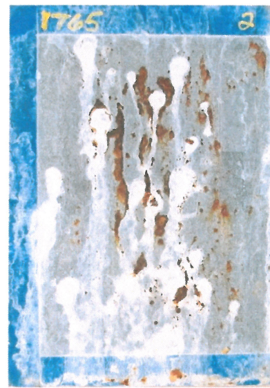
HDG G30 (.24oz/ft 2 ) Coated with InterCoat™ ChemGuard 315 (135mg/ft 2 )
