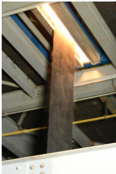
**The strip enters an infrared curing oven which, with temperatures between 140 and 300 degrees Fahrenheit, is energy efficient.**
