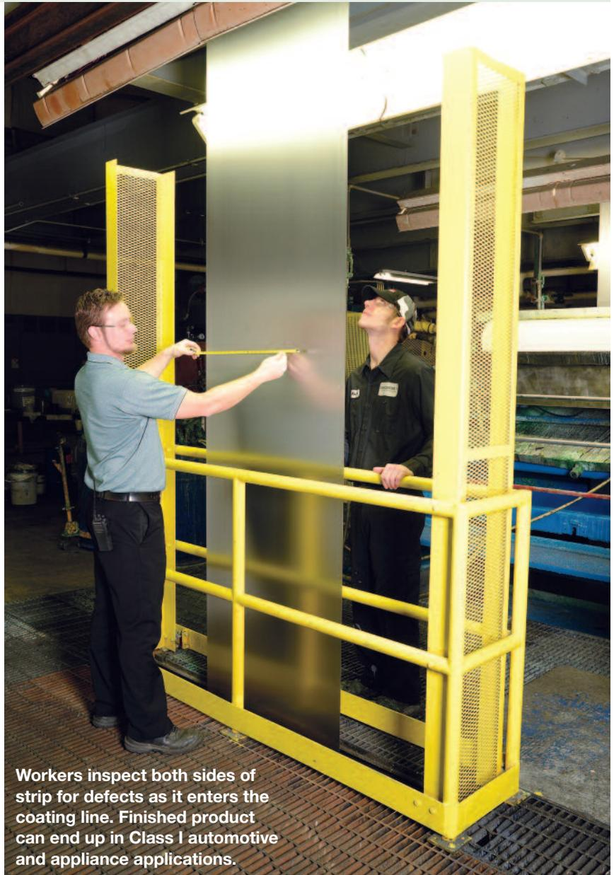
Workers inspect both sides of strip for defects as it enters the coating line. Finished product can end up in Class I automotive and appliance applications.
