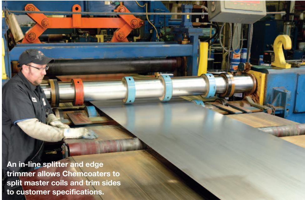
**An in-line splitter and edge trimmer allows Chemcoaters to split master coils and trim sides to customer specifications.**
